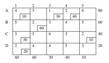
The minimum transportation cost associated with this solution is  $Z = \$(4 \times 10 + 1 \times 30 + 2 \times 40 + 2 \times 60 + 3 \times 30 + 2 \times 10 + 2 \times 20)$  = \$ (40 + 30 + 80 + 120 + 90 + 20 + 40) = \$420 By applying Zero Suffix Method the allocations are obtained as follows:
